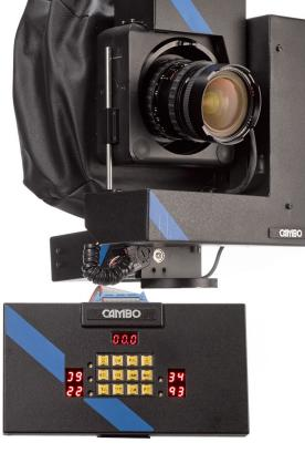
This fully motorised view camera was built in 1996 and shown on the PhotoKina that year.
